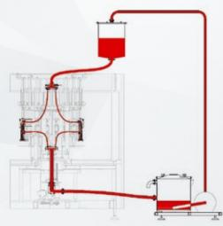
ENOBERG's RLF machine can be fully cleaned thanks to the dummy bottles, to the spray balls contained in the product tanks, to the piping system designed for recovering or recycling, depending on the needs, the washing solution, and to the Automatic cleaning phases (CIP).
