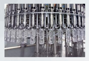
ENOBERG's EVF machine can be fully cleaned thanks to the dummy bottles installed next to each filling valve, and the spray ball contained in the product tank and to the piping system designed for recovering or recycling, depending on the needs, the washing solution.
