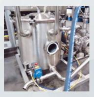
ready to be filled again. The machine can be configured for hot filling with recirculation system in order to guarantee a constant filling temperature and a return to pasteurizer of the product to be filled. Complete, versatile and easily serviceable, thanks to the filling valve entirely designed by Enoberg, it guarantees a high precision filling level.
