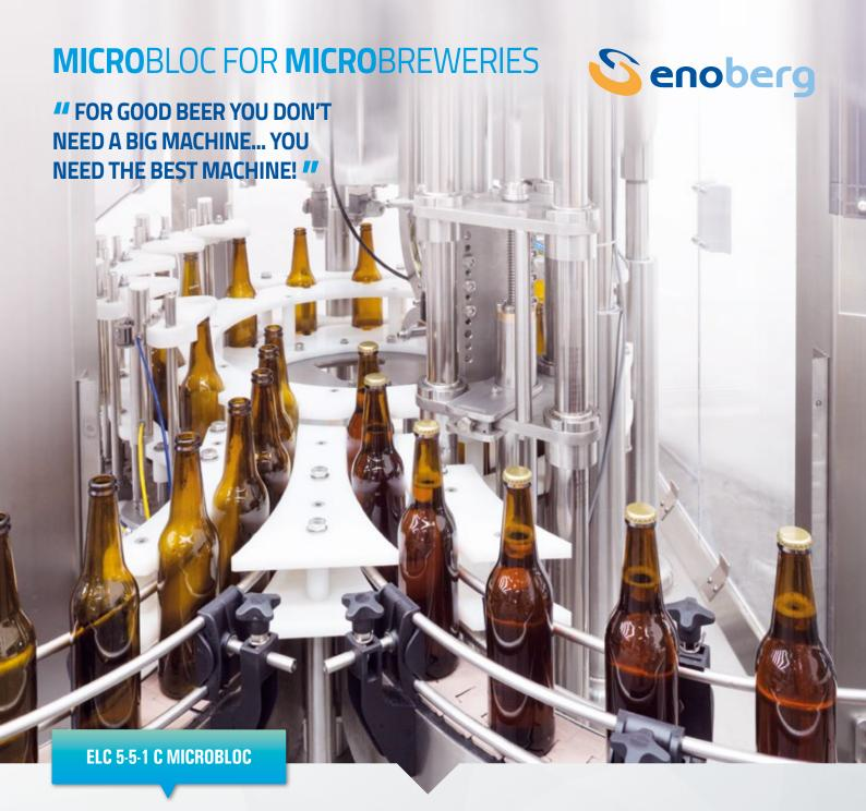
New microbloc for microbreweries complete with rinser, isobaric electro-pneumatic filler with double pre-evacuation system and single-head crown capper up to 1.000 bph for 0,33l format.
