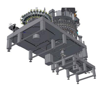
the filling chamber is completely isolated from the transimissions, which therefore do not come into contact with any type of liquid;
